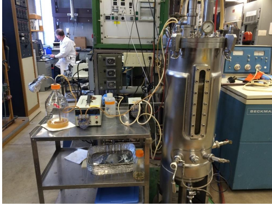
Figure 3.4 A 50 Liter sterilizable-in-place fermentor (Fermentation facility, ISU)
